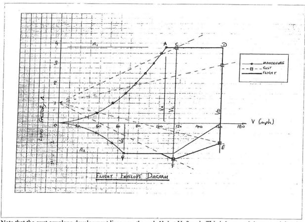
Note that the gust envelope development lines pass through 1'g' at V=0 mph. This is because it is assumed that the aircraft is accelerated by each gust from the 1'g' level flight condition.
