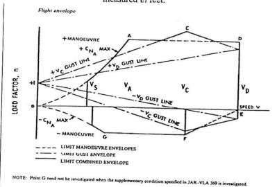
Both the manoeuvre and gust envelopes are calculated with the aircraft at its projected maximum all-up-weight. The exception to this would be an aerobatic aircraft where both the maximum aerobatic weight and maximum take-off weight would have to be considered.
